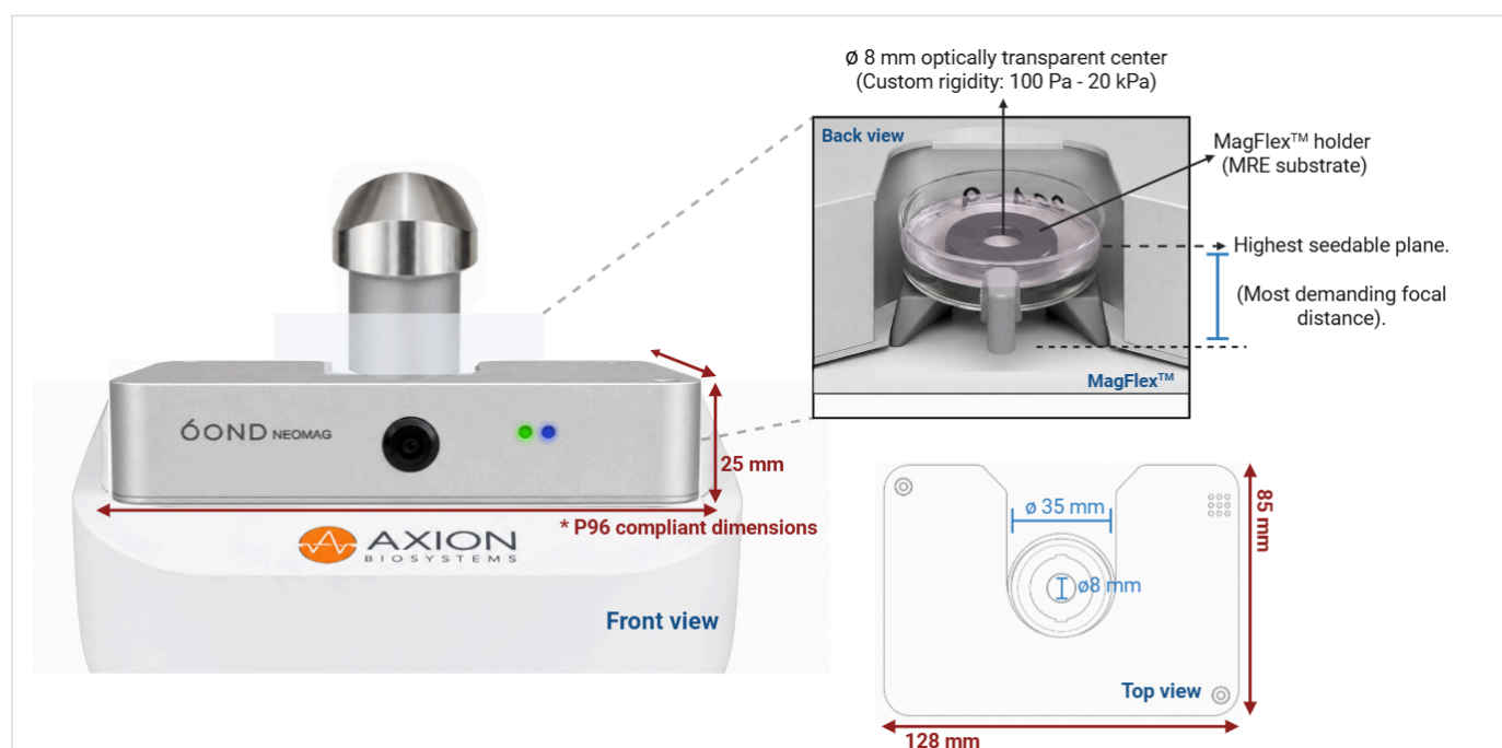
FIGURE 1. HARDWARE INTEGRATION AND MAGFLEX™ SET-UP
